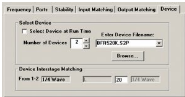
Figure 3: LINC2 amplifier synthesis device and interstage matching selection
